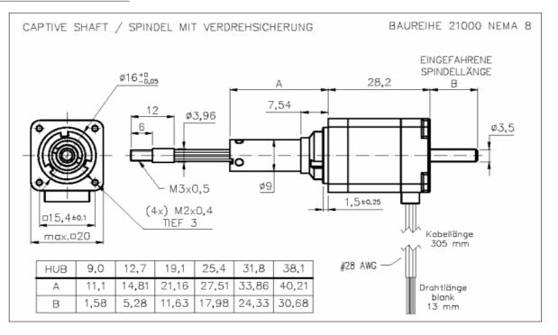
Max Linear Force Linear Stepper Motor can get is 30 N. Linear Motor give here very low Speed only :0,6mm/s.
