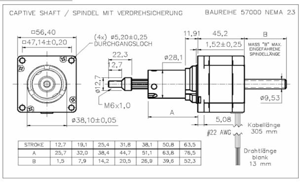
Max Linear Force Linear Stepper Motor can get is 700 N. Linear Motor give here very low Speed only :7mm/s.
